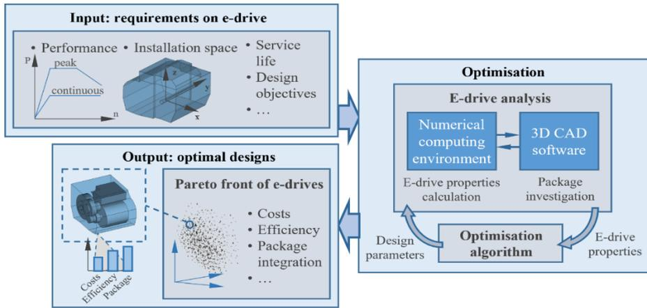
Figure 3: Simplified visualisation of e-drive optimisation process with OPED [8]
