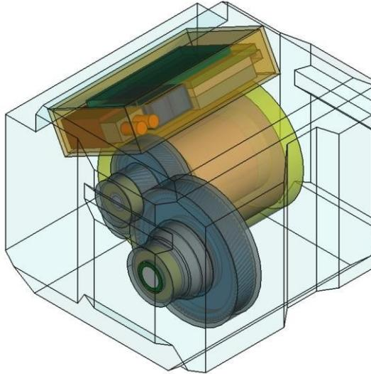
Figure 7: CAD visualisation of selected design solution inside the available installation space
