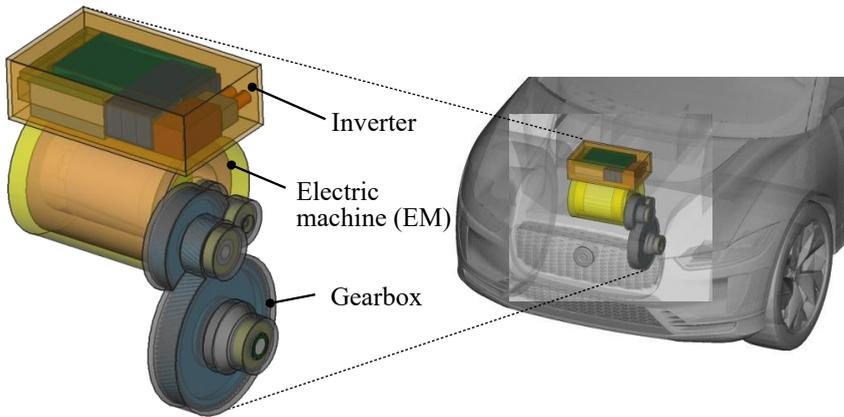
Figure 2: Visualisation of e-drive architecture; vehicle model from [5]
