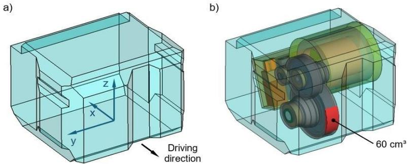
Figure 5: CAD visualisations of e-drive installation space: a) available space, b) package metric definition
