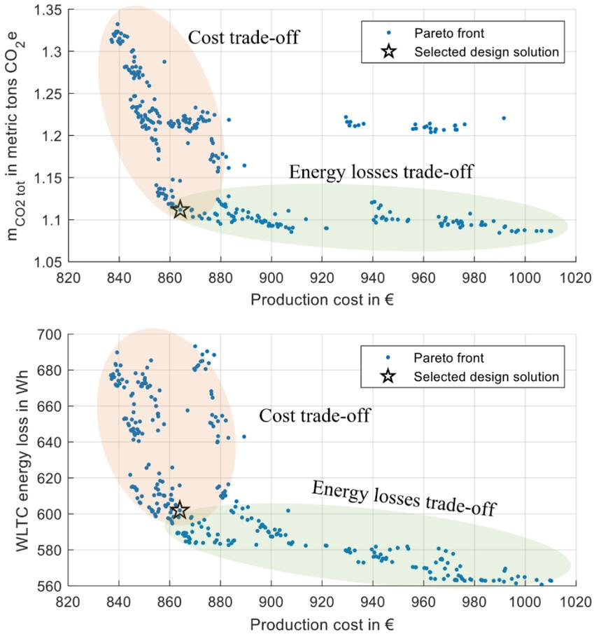
Figure 6: Projections of the obtained Pareto front approximation; only solutions that fit inside the installation space are shown
