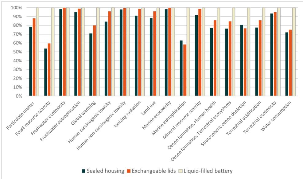
Figure 2. Relative environmental impact of the production phase for three battery pack designs, evaluated across multiple impact indicators - in relation to the highest contributor (set as 100%)
